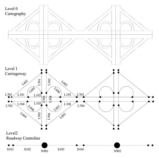
Figure 2. Abstraction of a flyover in a three-level network model.
